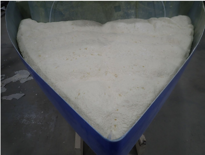
Figure 21. Flotation foam in the front part of the deck.
