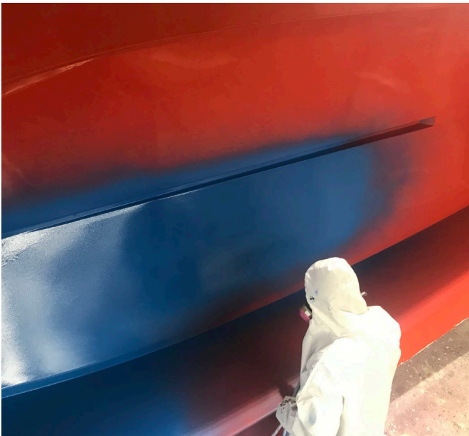
Figure 2. Application of gelcoat in the hull mould
