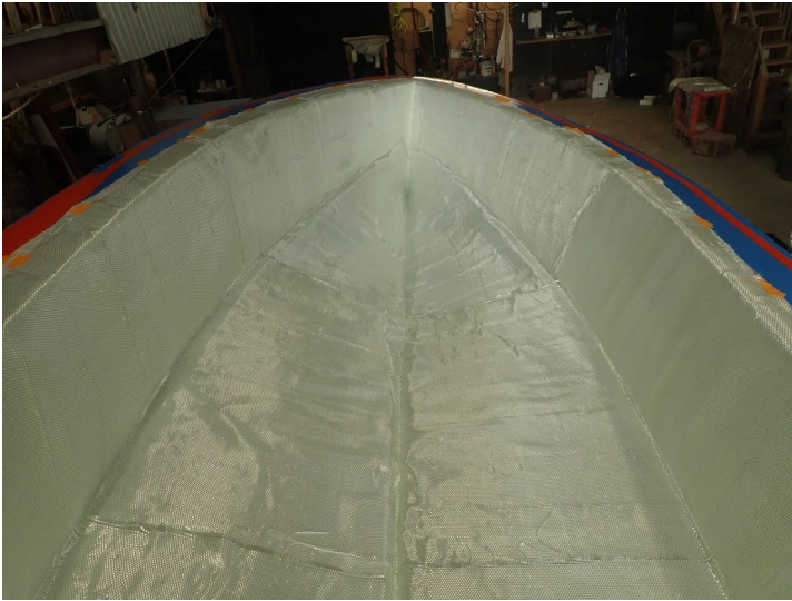
Figure 4. Positioning of the reinforcements in the hull mold
