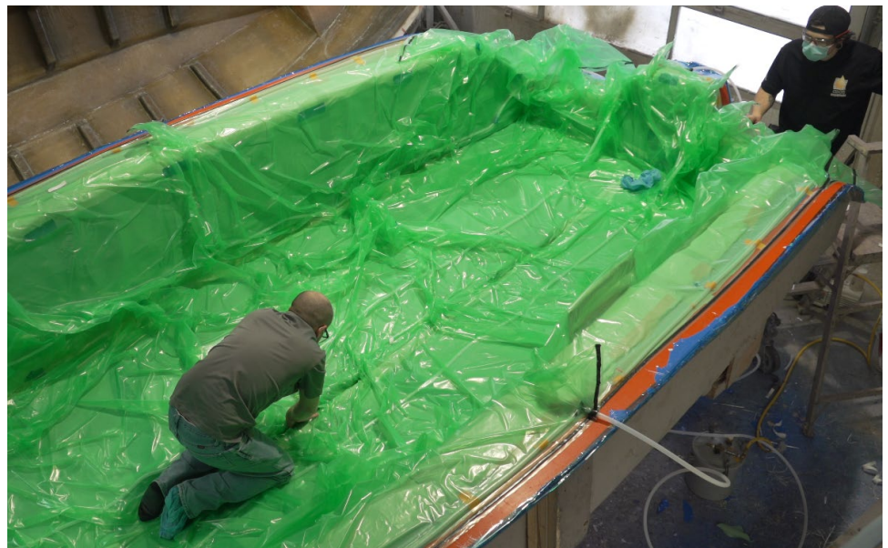
Figure 5. Positioning of release film, medium and infusion lines
