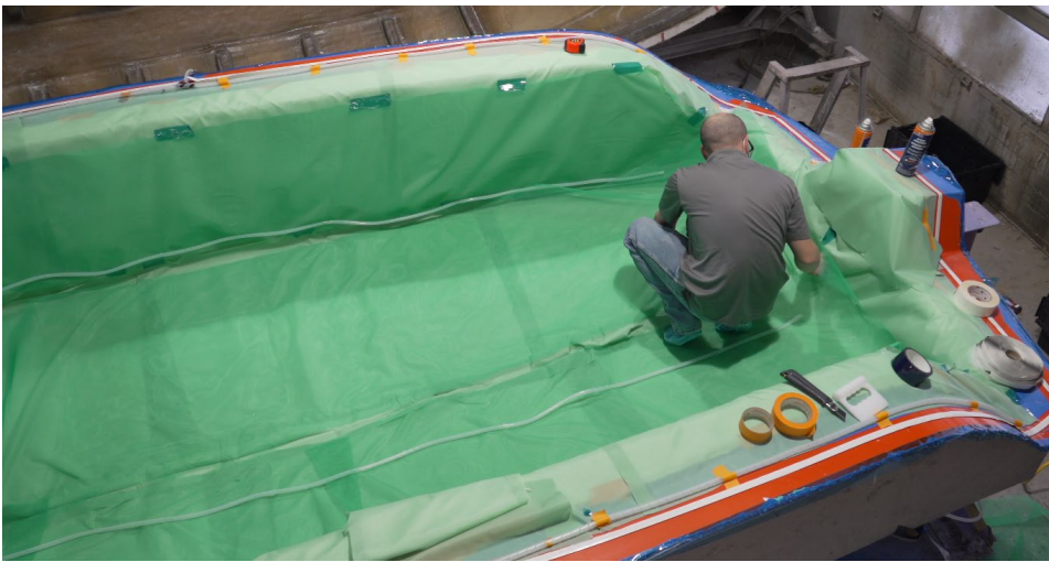
Figure 5. Positioning of release film, medium and infusion lines
