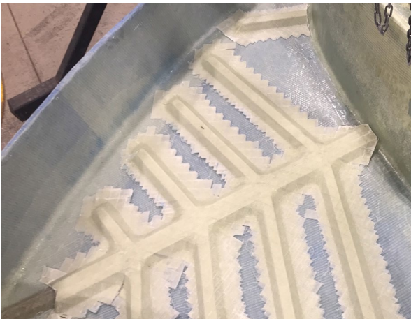
Figure 19. Gluing of the front sub-deck reinforcement
